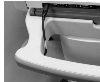
Not enough cable slack.
